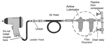
If an unusually long air hose is required, (over 8 metres), the line pressure or the hose inside diameter may need to be increased. The air hose must be rated at least 150% of the maximum operating pressure of the air tool.
